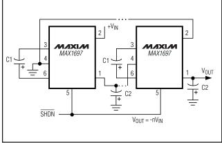
Figure 4. Cascading MAX1697s to Increase Output Voltage
