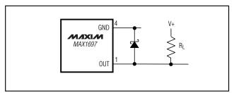
Figure 7. Heavy Load Connected to a Positive Supply
