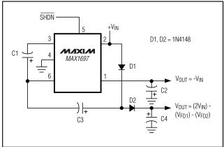
Figure 6. Combined Doubler and Inverter
