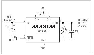
Figure 1. Typical Application Circuit
